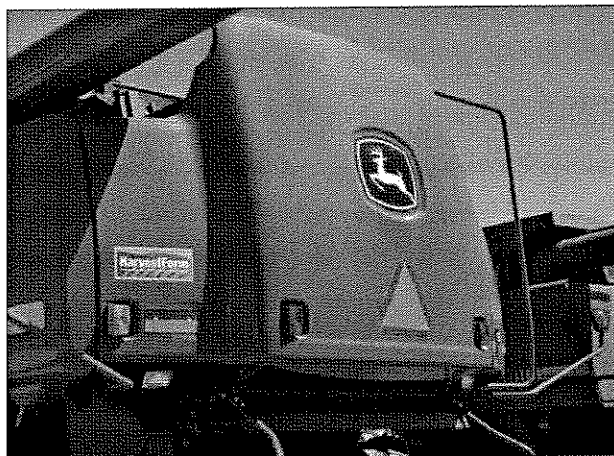
An Envirez thermoset plastic product. This product has various sheet molded applications and John Deere and Case New Holland are working to incorporate it in future moldings for tractors and combines.
